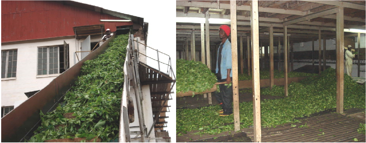
Fig. 6: Tea enters the withering room where moisture in the sprouts is dropped down to approximately 70%
