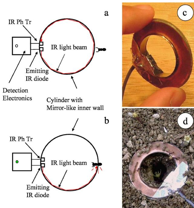
FIG. 2. (Color online) Description of the sensor that illustrates its functioning. (a) and (b) show a diagram to illustrate functioning. (c) and (d) show pictures of the ant activity sensor in the laboratory and set on a real nest exit, respectively.
