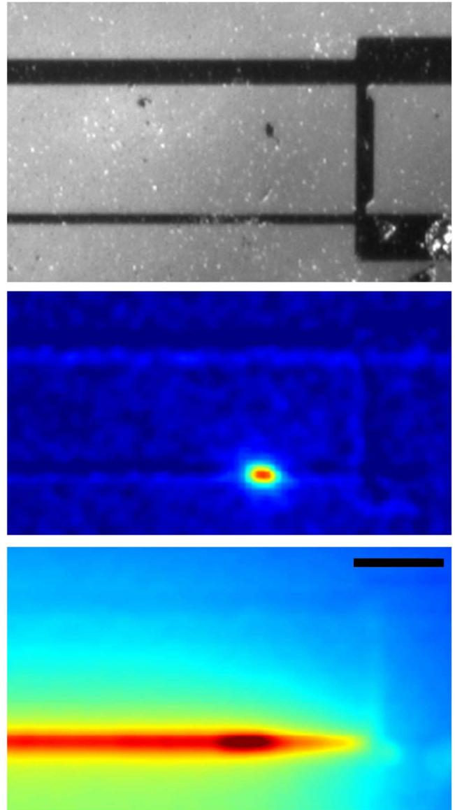
Fig. 7. Optical and thermal images of superconducting bridge III. The total transport current is 50 mA (middle) and 60 mA (bottom), but there is a second bridge in parallel. The temperature in the hotspot is measured to 94 K. The scale bar is 50  $\mu\text{m}$ .
