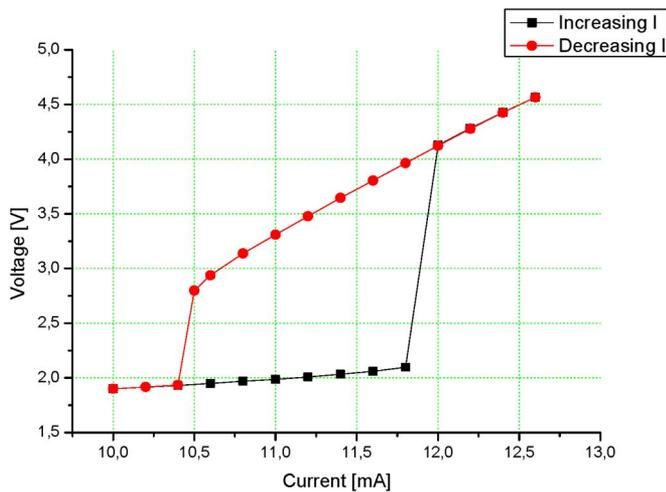
Fig. 6. Voltage versus transport current for superconducting bridge II. A hotspot is created at 12 mA and disappears at 10.4 mA.
