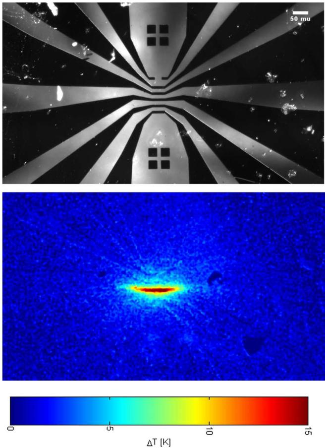
Fig. 5. Optical and thermal image of superconducting bridge II with 12 mA transport current.
