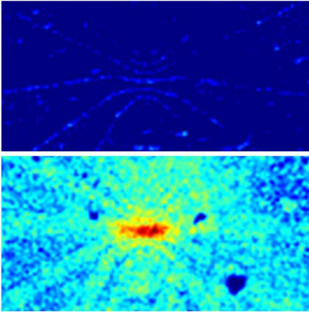
Fig. 8. Thermal images of a hotspot in superconducting bridge II initiated by an external applied magnetic field. The top image show the temperature for the two first seconds of transport current and the bottom image show from 3 second to 5 second. The hotspot is not started unless there is a magnetic flux density of 52 mT.
