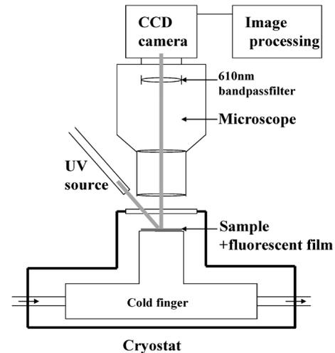
Fig. 1. Experimental setup for thermal imaging at cryogenic temperature. A fluorescent polymer film is deposited on the sample surface in advance.
