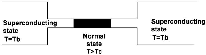
Fig. 2. Model for hotspot in superconducting bridge. The heat dissipation in the normal state raises the temperature above the critical temperature for the superconductor. The hotspot is therefore self-maintained.
