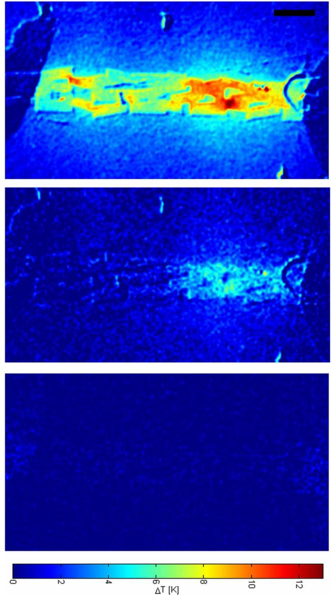
Fig. 4. Thermal images of superconducting bridge I with transport current. The transport current is 100 mA (top), 80 mA (middle) and 100 mA (bottom). The images show the bistable behavior of the bridge. The bridge is in normal or superconducting state for the same transport current at 100 mA. At 80 mA only part of the bridge is in normal state. The scale bar is  $500 \mu\text{m}$ .
